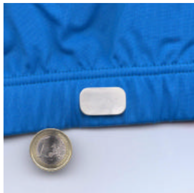
Fig. 6. Outside plate of an integrated thermogenerator, suited for an active area of 1 cm 2 .
