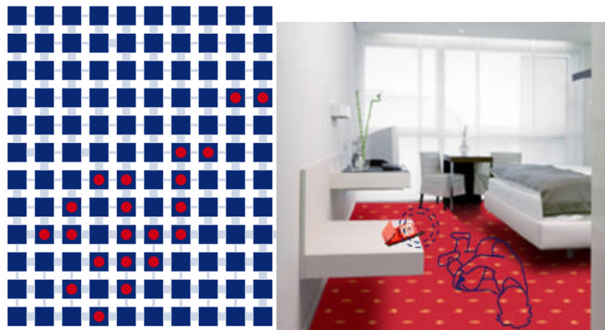
Figure 6 Sensor signals (left) derived from a person that lies on the smart carpet prototype like depicted in the right picture
