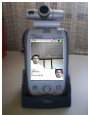
Fig.1. "Virtual Cameraman" on a PocketPC®: From a camera video the region containing the user's face is extracted and tracked over time. If only this portion is transmitted, a video-conferencing partner has the impression the camera is actively following the head. tracked from the camera image of the mobile
