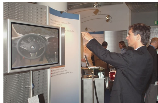
Fig.2. "Smart Cockpit": Using an image processing algorithm based on skin-color and movement speed, a user's pointing gestures are recognized robustly. In this example, interaction elements on a car dashboard can be controlled.
